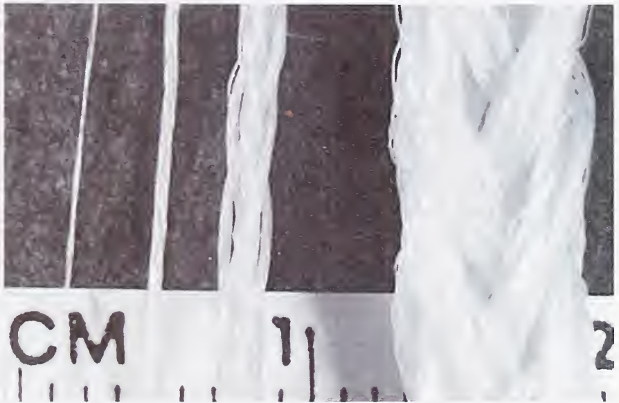
Collagen fiber and braided structures from collagen fiber: (a) single collagen fiber, (b) 8-ply collagen fiber braid, (c) 64-ply collagen fiber braid, (d) 512-ply collagen fiber braid.
